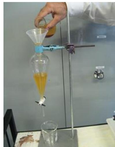
8. The mixture separates into layers. The glycerol from the vegetable oil sinks to the bottom while the biodiesel floats on top.
