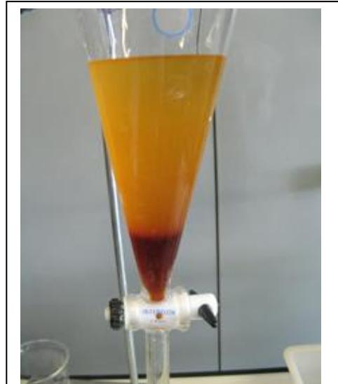
Figure 1 – the mixture containing biodiesel after settling.
